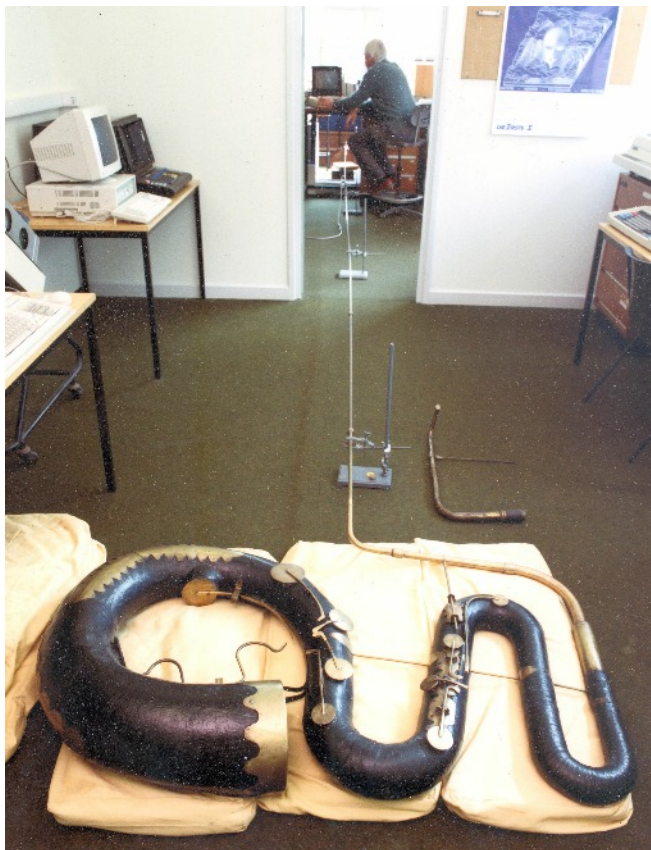
The Anaconda in the laboratories of the University of Surrey in 1988. The technique of acoustic pulse reflectometry requires the attachment of an initial cylindrical tube that is at least as long as the object to be measured. The experimenter in the control room is Philip Drinker; the original crook is lying on the floor.
