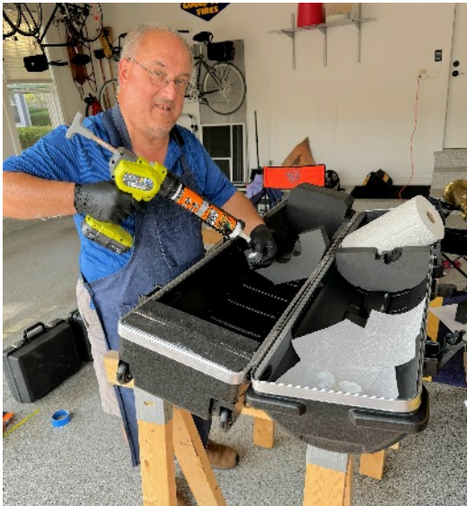
Paul Schmidt applies adhesive to foam blocking in Doug Yeo's new ophicleide road case
