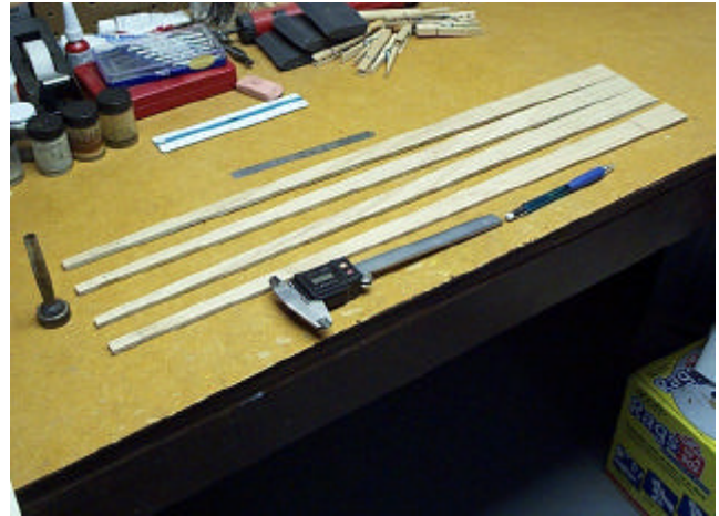
the four trapezoids after cutting them out from the plywood sheet
