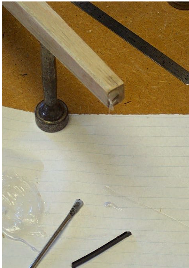
filling small end of bore with epoxy
