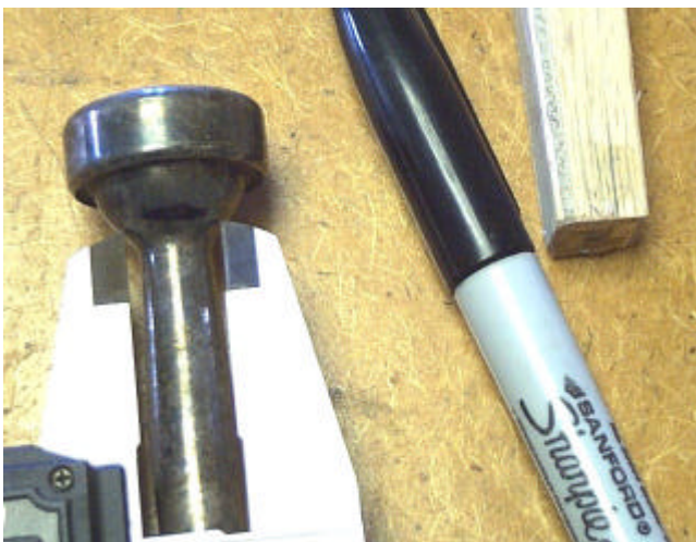
mouthpiece marked for cutting (see black mark near points of caliper)
