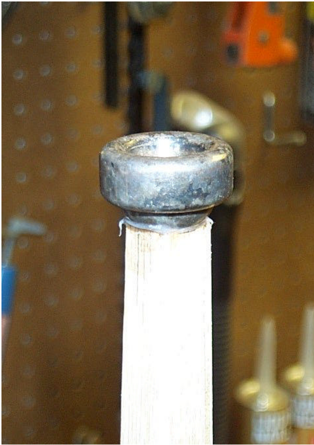
mouthpiece glued to wooden tube
