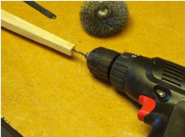
drilling out excess glue at small end of bore
