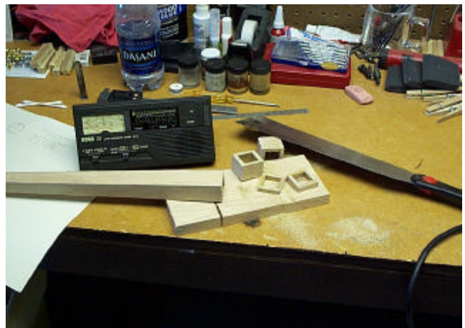
tuning the tube by trimming large end
