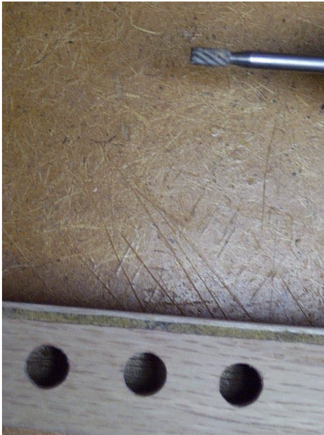
closeup of rotary bit used to undercut finger holes
