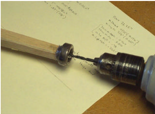
drilling out mouthpiece throat to remove excess epoxy
